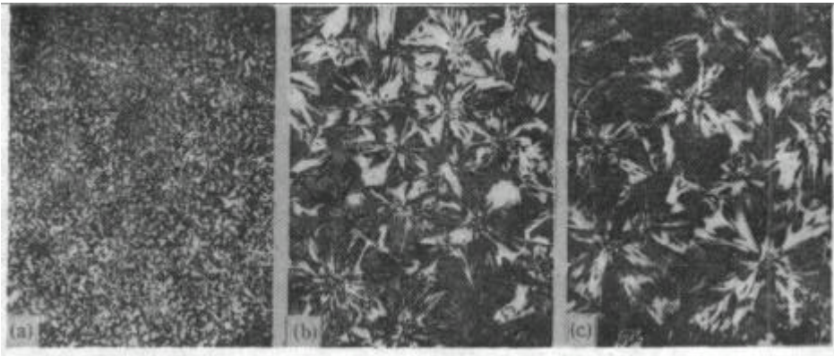
Fig. 8 Optical micrographs of L series samples crystallized at 288.2K, (a) L0; (b) L1; (c) L2
